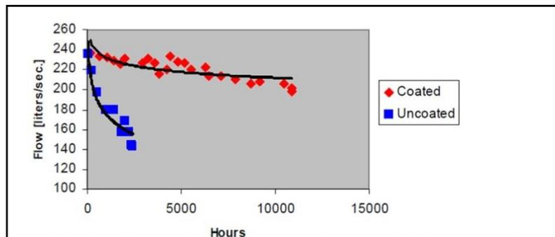
Figure 5: Flow rate as function of hours of service for Sulzer HPH 54-25 6-stage pump
