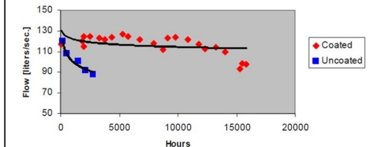
Figure 6: Flow rate as function of hours of service for Sulzer HPH 32-17½ 9-stage pump
