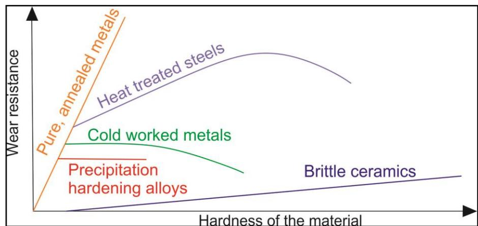
**Figure 2: Wear resistance as a function of hardness for several classes of material.**
