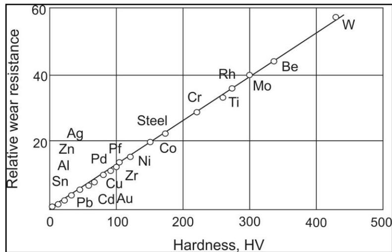
**Figure1: Abrasive wear resistance as a function of hardness for annealed un-alloyed metals and steel.**
