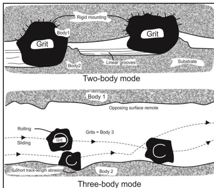
Figure 4: Schematic illustration of 2-body (top) and 3-body (bottom) abrasive wear.
