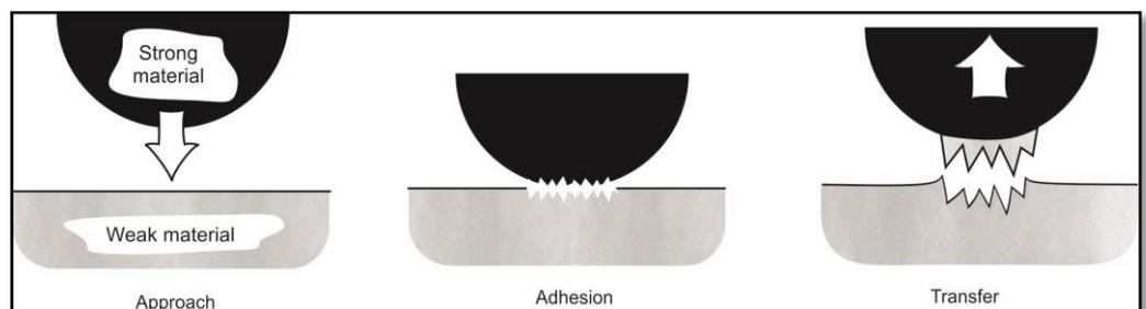
**Figure 3: Schematic illustration of adhesive wear.**
