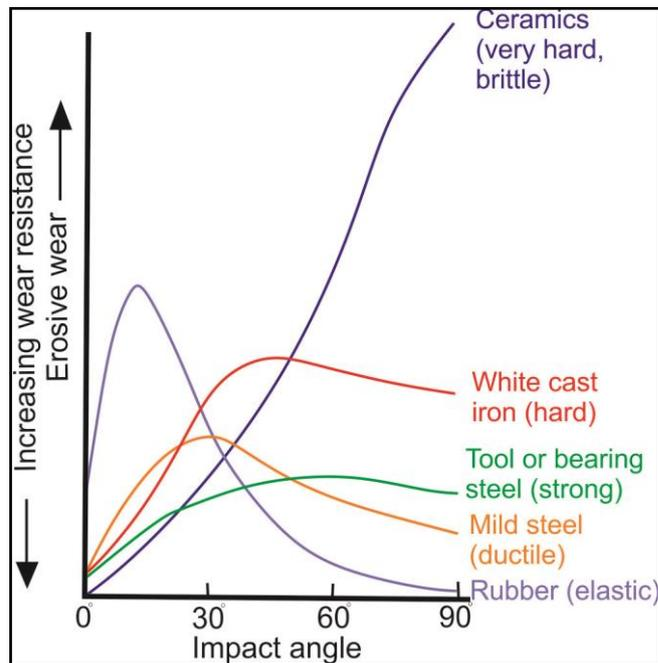
**Figure 6: Effect of impact angle on the wear resistance and erosive wear of different types of materials.**
