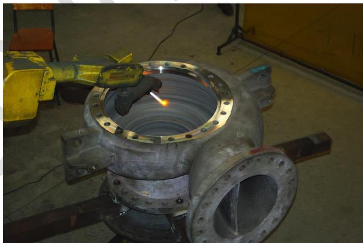
Figure 1: Pump casing - thermally sprayed with the HVOF process
