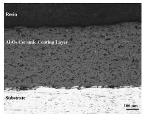
Figure.2. Mechanical Bond
