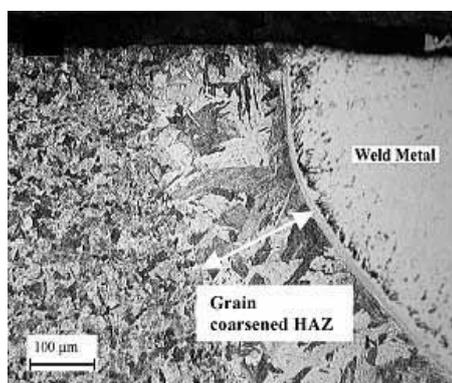
Figure.1. Metallurgical Bond
