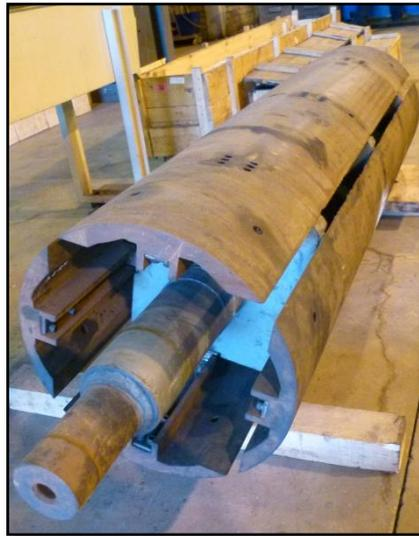
Figure 2a: Segments for coiling mandrel before coating
