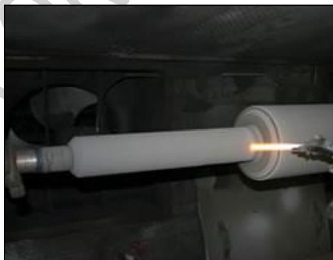
Figure 3: Furnace rolls coated with NiCr-Cr<sub>3</sub>C<sub>2</sub>
