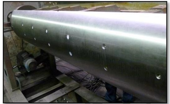
Figure 2b: Segments of coiling mandrel after coating
