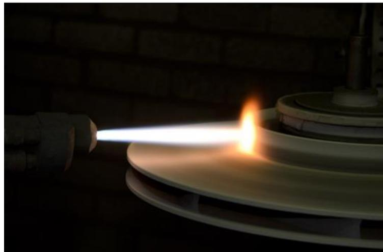
**Figure 2: Pump impeller - thermally sprayed with the HVOF process**
