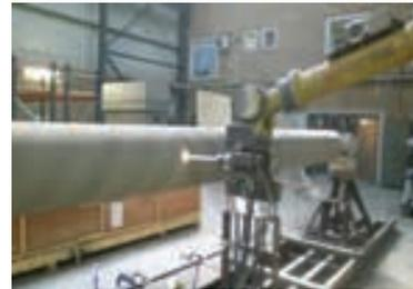
Figure 5: An HVOF chrome carbide, nickel chrome coating being applied to the length of the rod.
