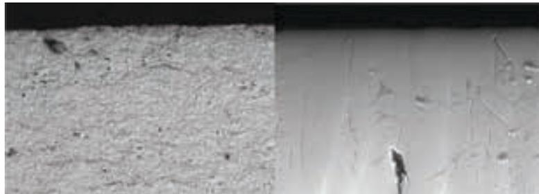
Figure 2: Comparative surface micrographs of a thermal spray coating (left) and a 'mud-cracked' hard chrome plated surface (right).
