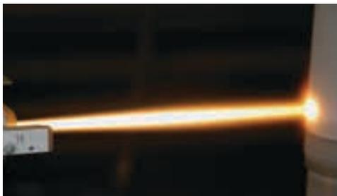
Figure 1: An HVOF thermal spray coating being applied to a hydraulic component.
